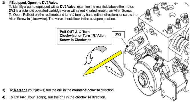
5) When Manual Override is complete, return the cartridge valve(s) And DV2 (if equipped) to the Normal Positions. Reinstall Black Plastic Cap/Silver (Foil) Seal on motor.
