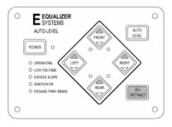
**Power OFF:** Press and release the POWER keypad button.
